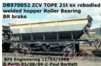
DB970052 ZCV TOPE 21t ex rebodied welded hopper Roller Bearing BR brake RFS Engineering 11/03/1988 Perth 01/08/99 © Paul Bartlett ZCV Tope DB970052 at Perth, 1st August 1989. Paul Bartlett
