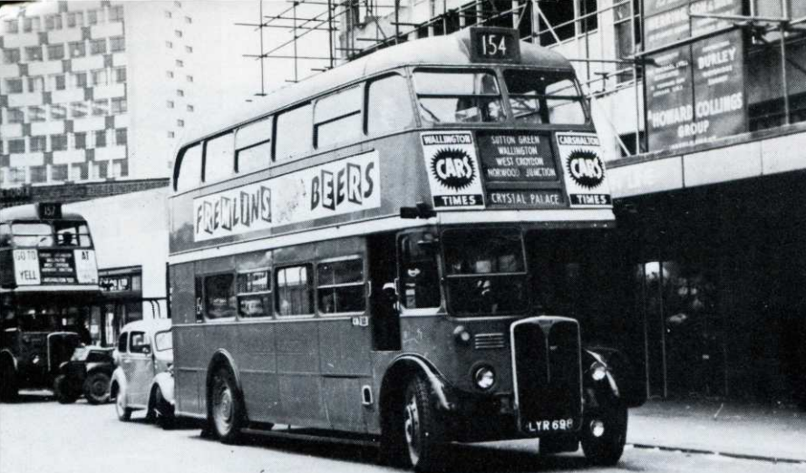
The new office block goes up over Morden Station alongside the newly established stand for route 154. Carshalton's RT2714 has an RT3 body, as did many used for this conversion. Another Carshalton RT3 on route 157 stands further back. K. W. Glazier
