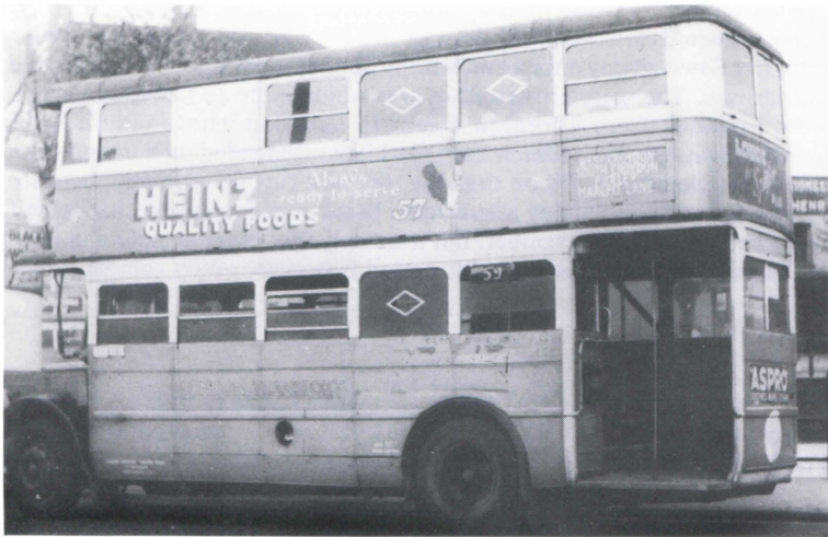
This photo of TC's ST26 at Thornton Heath Pond shows the wartime window netting and boarded window (glass was not easy to acquire) on route 59B. W.J. Haynes
