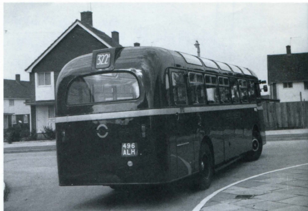
The total absence of Chiswick influence in the Willowbrook body is very apparent in these views of RW2 at Warners End on the first Sunday in service of the class. Note the unique arrangement for the rear route number blind, a solution not pursued on subsequent single-deckers. K. W. Glazier
