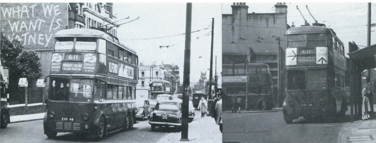
The 611 had a delayed introduction in June 1939 and was now withdrawn ahead of other services in the area. The BRCW-bodied J3 class of AECs was fitted with run back and coasting brakes to accord with a police regulation requiring their use on Highgate Hill. Only two of the class were to survive the withdrawal of route 611. No. 1048 is seen starting the ascent at Archway, a few weeks before the changeover . . . Michael Dryhurst . . . and the same vehicle stops at the mandatory Bus Stop to engage the coasting brakes before descending the hill. This bus stop was unique in London in being of internally illuminated glass, to make it stand out after dark. C. Carter
