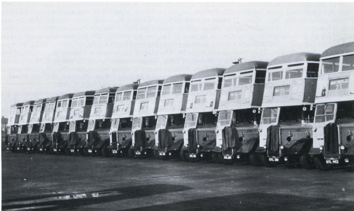
This line up of Gs at Barking illustrates the different dome and cab window styles utilized by the various body builders in their varying interpretations of the basic austerity design. Malcolm E. Papes
