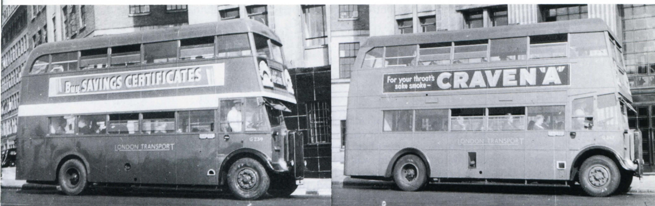
Left: Photographs of Guys operating from Victoria garage are rare since the class survived there for a matter of months before being sent onto Enfield in exchange for STLs. G239 bodied by NCME and in a brown and cream livery, is seen on route 77A. Right: The angular Massey body of G267 contrasts with the slightly more streamlined interpretation of austerity specification by NCME. The livery is two shades of brown and the vehicle is operating on route 77A from Victoria garage. Malcolm E. Papes
