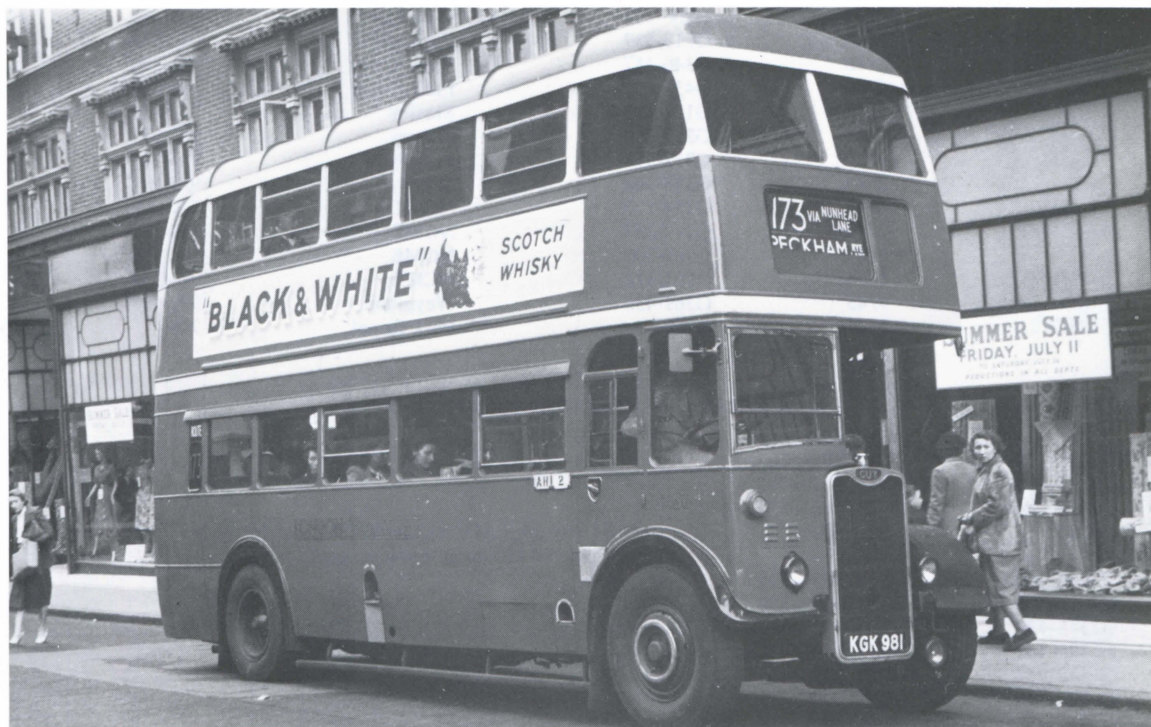
G436 was the lone 4G13 delivered in 1950 with Guy bodywork. It spent the first part of its life operating route 173 at Old Kent Road but by July 14th 1952 when this photograph was taken it was working the route from Nunhead. The body is to Park Royal design and is similar to many supplied by Park Royal to Provincial operators. Alan B. Cross
