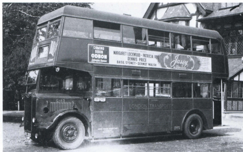
Delivered to Barking in an all brown livery Massey bodied G183 is seen at Chingford (Royal Forest Hotel), the terminus of route 145. No side blind is carried though a route number stencil is provided in the nearside rear window. Alan B. Cross
