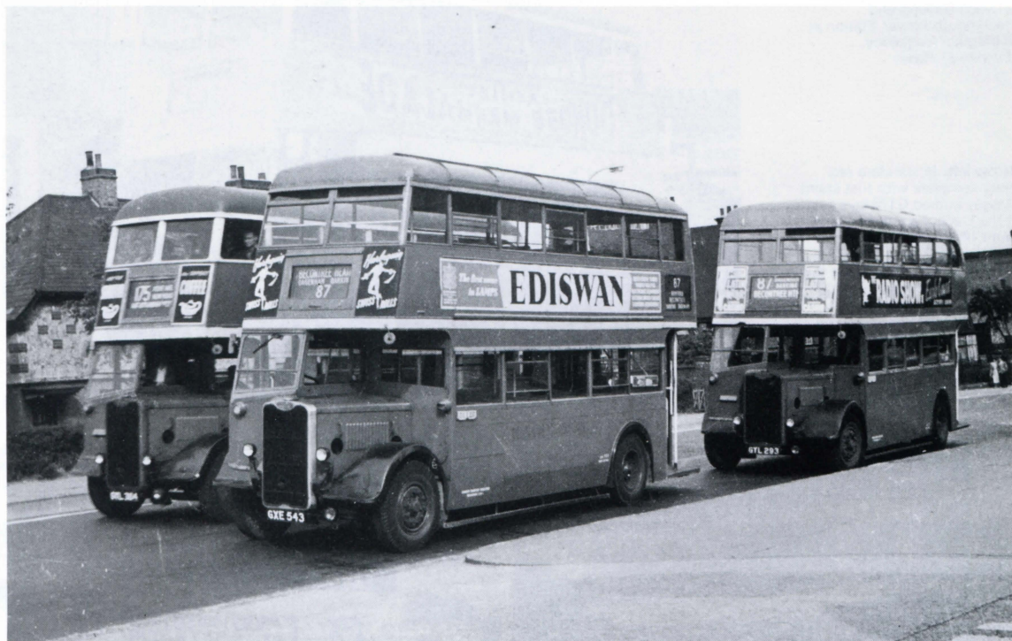
This view of G103 (Park Royal), G225 and 154 (both NCME) at Becontree Heath provides an interesting comparison of the frontal treatment provided by the two bodybuilders. The different blind layouts will be noted together with the fact that part of the destination screens of certain vehicles were painted out to accommodate the blinds. Brian Bunker
