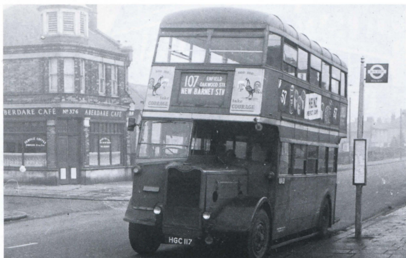
As part of a batch whose delivery began in December 1945 G338 was an example of a Park Royal bodied Guy with a number of features indicating a slight relaxation of the austerity rules. A side blind was fitted as new. Route 107 had a complicated series of workings, New Barnet Station being a Sunday morning terminus. Alan B. Cross
