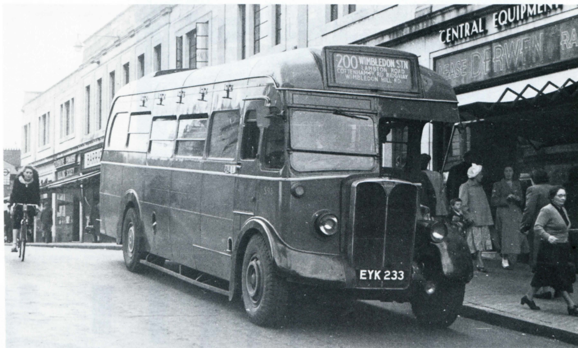
Top left: Between 1936-1952 the usual allocation for route 200 from AL was the 5Q5 as is shown here by Q125. These buses with all-metal Park Royal 37-seat bodies performed sterling service even in their later days. The position of the underfloor engine can clearly be seen allowing a genuine front entrance at a time when such a design was considered unacceptably avant garde. Malcolm E. Papes. Top right: Those with long memories might well recall that LT six-wheelers were regular to the 200 before the 5Q5s appeared but LT1019 had probably been loaned to AL from its usual home at Sutton (A) when the former were in short supply. The vehicle lasted until June 1952 and displays the usual lazy blind. J.H. Aston. Above: In this July 1952 view T598 (AL) is also helping out on the route. The vehicle started life as a Green Line coach in August 1938 but was converted to an ambulance for the duration of the War. In September 1951 it was painted red and converted to a bus; this included locking the doors open as they were not otherwise considered safe by the Metropolitan Police. These buses were classified 10T10. The full blind is notable. Alan B. Cross
