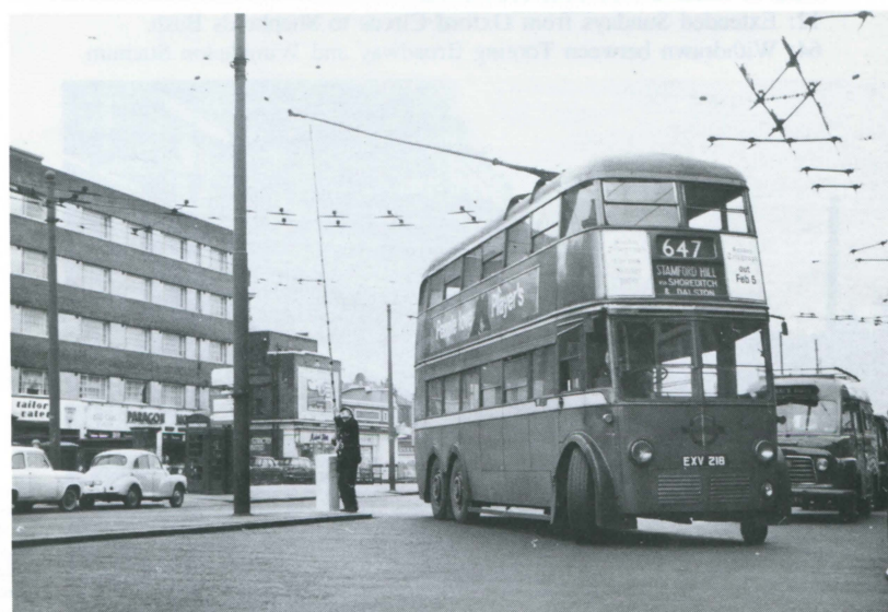
Right: K1 1114 on route 643 sweeps into Stamford Hill on the through wires, having just crossed the terminal loop which runs into a siding for layover buses. Between the trolleybus and the traction pole on the centre island can be seen the junction wiring for the turning loop from the other direction. On the same pole is the bamboo pole used for dewiring and rewiring . . . which was especially useful when a dewirement occurred. Such was the fate of K2 1218 on 30th January, no doubt to the dismay of the drivers of the other vehicles held up by the immobilised trolleybus. Michael Dryhurst/A.J. Wild.
