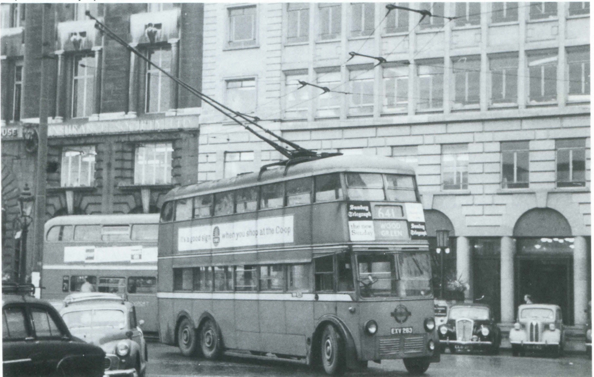
Above left: STAGE 11 Some shortworkings saw spasmodic use, and that at Downham Road, Kingsland Road was rarely used. On the last day, 18th July 1961, however, 1214 was curtailed there; because of its infrequent use it entailed a pole swap instead of a frog. This was an awkward procedure here due to fouling the zebra crossing, there being only a short section of adjacent loop wire. In fact on this occasion, which was the last ever use of these wires, the second pole would not swing over and the photographer had to complete the swap as the driver moved 1214 up a few feet. The list of approved turning points for this particular location restricted use here from 6.00–9.20 am and 6.00–8.00 pm though this photograph was taken outside these hours. Hugh Taylor. Above right: STAGE 12: 1515 departs from Finchley depot on the afternoon of the last day, 7th November 1961. Transferred PR/FY it now moves FY/FW and will work until the last day of London Trolleybus operation. 1515 halts at the top of Woodberry Grove as a ferryman goes for the frog. Finchley sent many of their vehicles away with their blinds correctly showing blank and 'Private'. At other depots they either took the blinds out or left them in with various permutations showing. Tony Belton. Below: It's the last of trolleybuses operating at Moorgate, but this does not deter the driver of 1263 from losing his poles in Finsbury Square. Peter Moore
