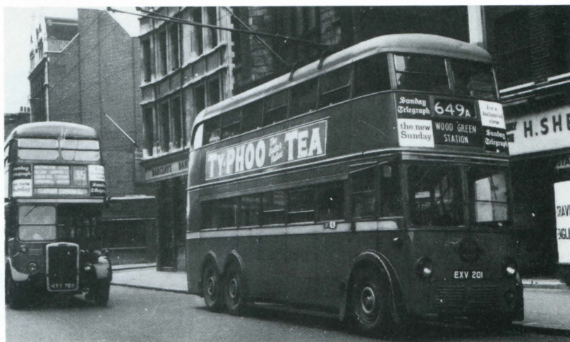
Right: Route 649A ran only on Sundays – the only route to do so. 1201 is now preserved by the London Trolleybus Preservation Society at Carlton Colville, but is seen here at Liverpool Street. Note the two banks of flutes in the valance which were to be found on some of the K class vehicles. Photomatic
