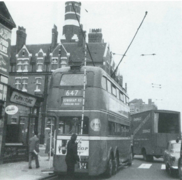
Above left: STAGE 11 Some shortworkings saw spasmodic use, and that at Downham Road, Kingsland Road was rarely used. On the last day, 18th July 1961, however, 1214 was curtailed there; because of its infrequent use it entailed a pole swap instead of a frog. This was an awkward procedure here due to fouling the zebra crossing, there being only a short section of adjacent loop wire. In fact on this occasion, which was the last ever use of these wires, the second pole would not swing over and the photographer had to complete the swap as the driver moved 1214 up a few feet. The list of approved turning points for this particular location restricted use here from 6.00–9.20 am and 6.00–8.00 pm though this photograph was taken outside these hours. Hugh Taylor. Above right: STAGE 12: 1515 departs from Finchley depot on the afternoon of the last day, 7th November 1961. Transferred PR/FY it now moves FY/FW and will work until the last day of London Trolleybus operation. 1515 halts at the top of Woodberry Grove as a ferryman goes for the frog. Finchley sent many of their vehicles away with their blinds correctly showing blank and 'Private'. At other depots they either took the blinds out or left them in with various permutations showing. Tony Belton. Below: It's the last of trolleybuses operating at Moorgate, but this does not deter the driver of 1263 from losing his poles in Finsbury Square. Peter Moore
