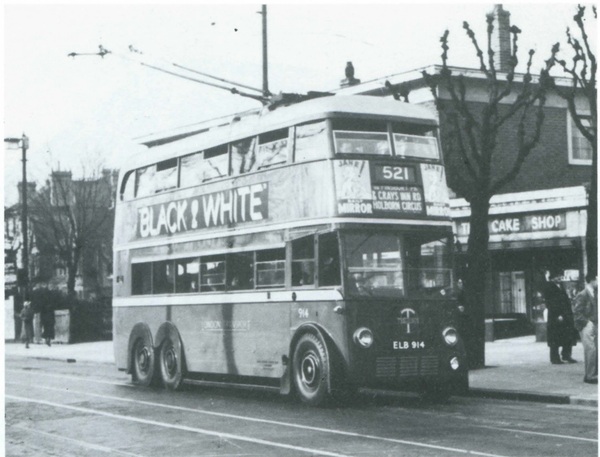
914 at Bounds Green illustrates the early days of trolleybus operation. Note the use of an offside route holder, the silver roof, single running plate and the same size via point as terminal point on the destination blind. Photomatic
