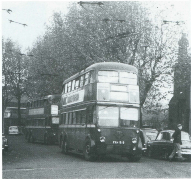
Above left: STAGE 11 Some shortworkings saw spasmodic use, and that at Downham Road, Kingsland Road was rarely used. On the last day, 18th July 1961, however, 1214 was curtailed there; because of its infrequent use it entailed a pole swap instead of a frog. This was an awkward procedure here due to fouling the zebra crossing, there being only a short section of adjacent loop wire. In fact on this occasion, which was the last ever use of these wires, the second pole would not swing over and the photographer had to complete the swap as the driver moved 1214 up a few feet. The list of approved turning points for this particular location restricted use here from 6.00–9.20 am and 6.00–8.00 pm though this photograph was taken outside these hours. Hugh Taylor. Above right: STAGE 12: 1515 departs from Finchley depot on the afternoon of the last day, 7th November 1961. Transferred PR/FY it now moves FY/FW and will work until the last day of London Trolleybus operation. 1515 halts at the top of Woodberry Grove as a ferryman goes for the frog. Finchley sent many of their vehicles away with their blinds correctly showing blank and 'Private'. At other depots they either took the blinds out or left them in with various permutations showing. Tony Belton. Below: It's the last of trolleybuses operating at Moorgate, but this does not deter the driver of 1263 from losing his poles in Finsbury Square. Peter Moore
