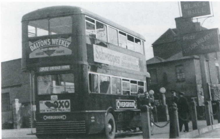
The Lances soon assumed a mainly red livery and standard front and rear indicators as can be seen in this view of D4 on route 307 at Whetstone (Black Bull) terminus. The heavy rear bumper did not last long. The rear number plate is now in the conventional London position instead of being above the rear window. W. J. Haynes
