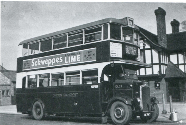
In October 1934 DL29 and two others from Ambassador arrived at PB allowing the Dennis H open-top buses to be transferred to Putney Bridge (F). The new route number 134 is carried and Victoria Coach Station is shown as the ultimate destination. The bus was a bit of a compromise: the staircase was appropriate to an open-staircase version, and the enclosed rear end looked like an afterthought. D. W. K. Jones
