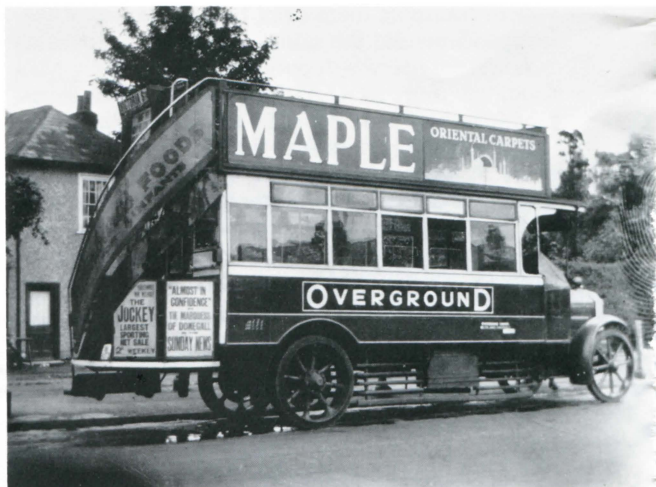
Above left: The last Leyland to be delivered to Overground whilst independent was YP 5287 (33) and was only a year old when photographed at Hadley on 15th July 1927. This view shows that the vehicle probably received a Dodson body of an earlier date as is evidenced by the inverted L-panel at the rear. W. Noel Jackson Above right: Still retaining the original domed metal mudguards of 1924 Dennis XW 5379 (17) was photographed in Hadley in 1927. Many of these had been replaced by plain bentwood guards after numerous encounters. D. W. K. Jones
