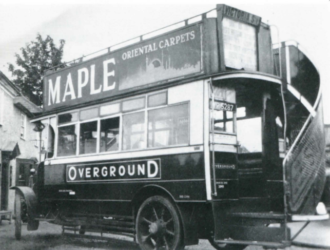
Above left: The last Leyland to be delivered to Overground whilst independent was YP 5287 (33) and was only a year old when photographed at Hadley on 15th July 1927. This view shows that the vehicle probably received a Dodson body of an earlier date as is evidenced by the inverted L-panel at the rear. W. Noel Jackson Above right: Still retaining the original domed metal mudguards of 1924 Dennis XW 5379 (17) was photographed in Hadley in 1927. Many of these had been replaced by plain bentwood guards after numerous encounters. D. W. K. Jones
