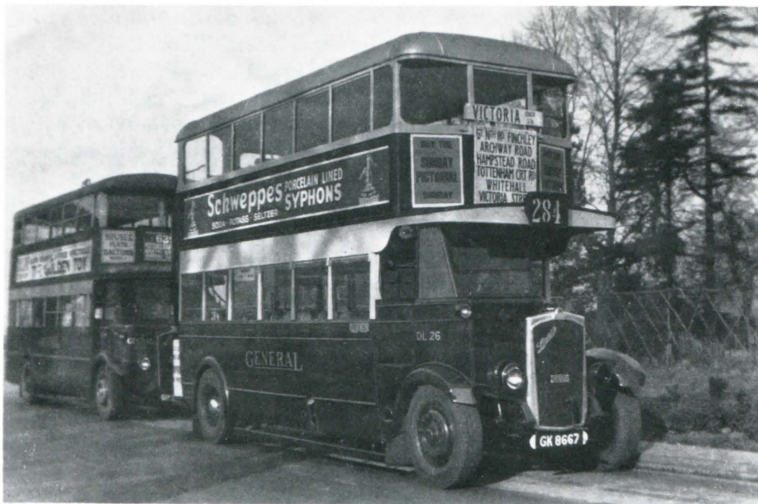
An early ex-Independent acquisition was DL26, ex-Claremont, which arrived at PB and started work on the 284 on 11th February 1934. It was fully 'Chiswicked' even to the white-tipped number plates and was given a bright metal radiator shell, a feature which became widespread on the Lances. Some comparisons can be made with the Lances on the 629 behind. D. W. K. Jones
