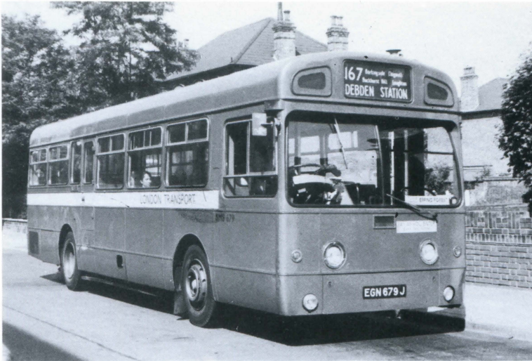
Here we see an example of the Swift family chosen for the single manning of route 167. These buses were three feet shorter than the Merlins but being relatively underpowered they thrashed along at only a modest pace. SMS679 (L) lays over at York Road, Ilford and carries a yellow sticker proclaiming operation to Epping Forest – in the case of the 167, a very debatable point. Malcolm E. Papes
